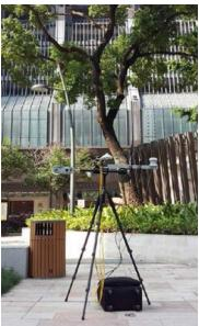
measure Short-wave and long-wave radiation
