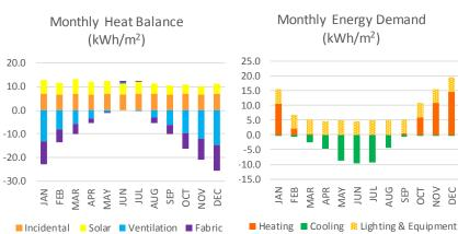
Step 2. Passive design (89.8kWh/m<sup>2</sup>/year)
