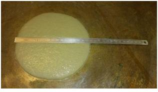
Flow test on shaking table
