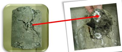
Formation of gel from oxidation of metallic aluminium
