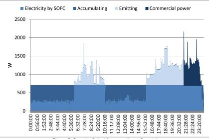
Figure 5: Supply of electric power (large 2peaks)
