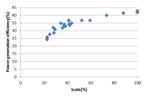
Figure 1: Power generating efficiency of SOFC
