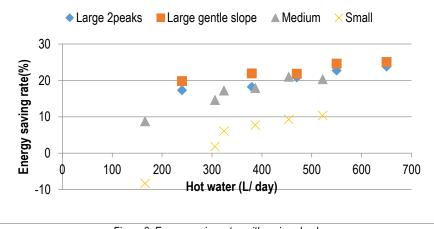
Figure 9: Energy-saving rates with various loads
