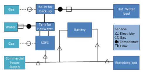
Figure 3: System of SOFC and battery
