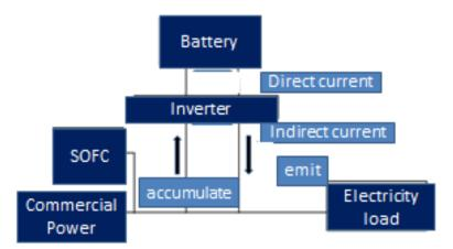
Figure 13: Mechanism of SOFC + battery system
